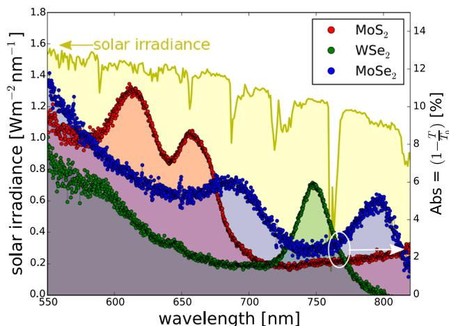
FIG. 1. Absorption in few-layer flakes of different TMDCs in comparison with the solar irradiance (AM1.5, yellow). The absorption is enhanced at the respective direct band gap energies. Of these three, MoSe<sub>2</sub> covers the broadest range in the absorption spectrum, starting at ~820 nm due to its small band gap, making it suitable for photovoltaic applications.
