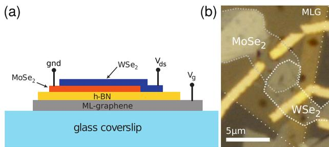
FIG. 2. (a) Schematic and (b) optical micrograph of the device showing the transparent glass substrate with a multilayer graphene and h-BN flake serving as the gate electrode and dielectric layer, respectively. On top of this stack, the MoSe<sub>2</sub> and WSe<sub>2</sub> flakes are transferred creating an overlapping junction. Metal contacts (Pd/Au) are added for electrical characterization.
