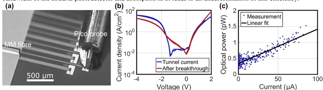
Fig. 2: (a) Photograph of LETJs. The Pico probe is used for electrical contact while the multimode (MM) fiber is used to extract the photons from the WGs. (b) IV curves of a broken (red) and unbroken (blue) tunneling junction. (c) Received optical power in the InGaAs photodiode versus the measured tunneling current.
