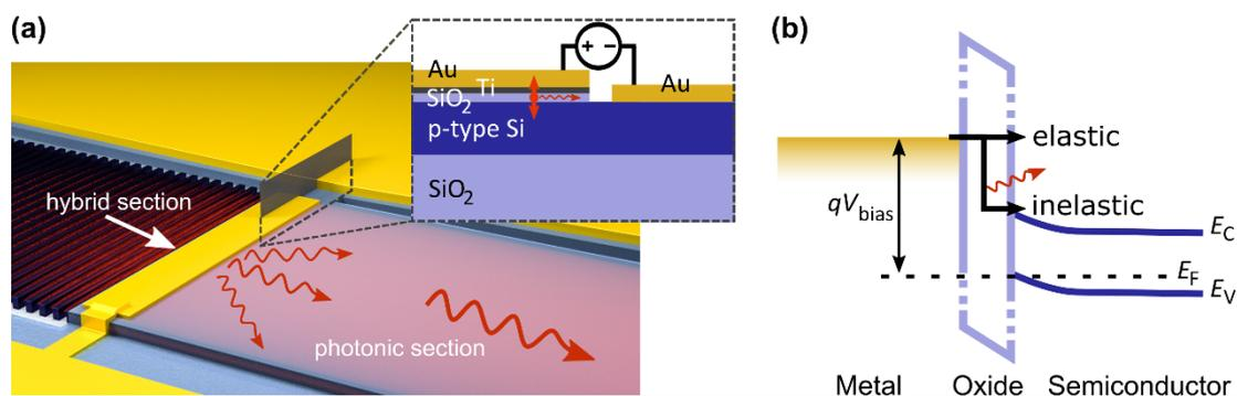
Fig. 1: (a) Rendering of a LETJ. Hybrid plasmonic modes are excited in the hybrid section and guided out in the photonic WG. The insert shows the cross-section (grey plane) through the structure. The emission is modeled as a dipole (red) perpendicular to the layer stack. (b) Band diagram of the MOS stack, showing possible elastic or inelastic tunneling pathways.
