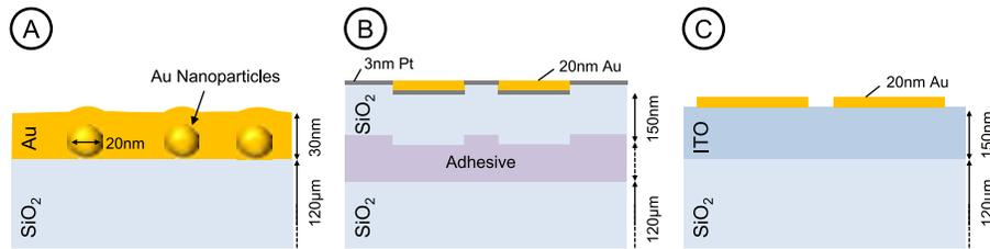
Fig. 1. Cross-sections of sample types A, B, and C as described in the text.
