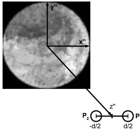
Fig. 5. The intensity distribution of light with 510 nm wavelength at the position of the fiber bundle source as measured by a camera. The diameter of the circular area is 0.62 cm. The shown coordinate axes were used in applying the van Cittert-Zernike theorem. The two circles represent the two pinholes at positions  $P_1$  and  $P_2$  of a Thompson-Wolf experiment where  $d$  is the center-to-center pinhole separation distance.
