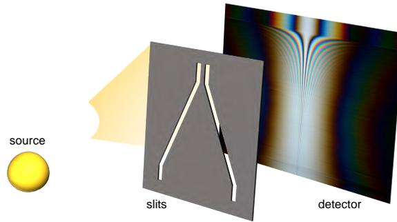
Fig. 1. A diagram (not drawn to scale) of the essential elements of the apparatus. Broadband light from an extended source passes through the non-parallel double slit aperture and generates an interference pattern on the detector plane.
