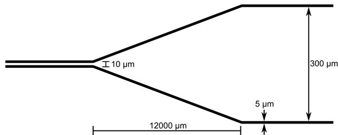
Fig. 2. A schematic (not drawn to scale) of the two-slit aperture used to measure coherence functions. The black lines represent transparent slits and white represents areas of high opacity.
