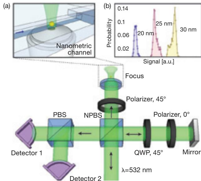
Dual-phase apparatus and histograms of particle-detection events. (a) A microscope objective focuses light onto a nanometric channel, and particles flow past. Scattered light is collected by a dual-phase interferometer. (b) Histogram showing results from three different immobilized particles.
