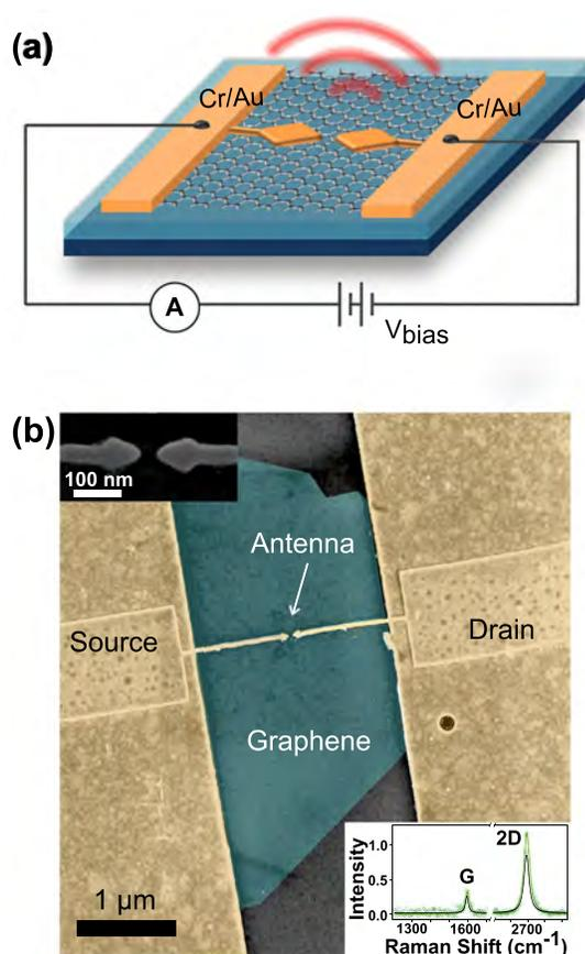
FIG. 1. (a) Illustration showing an antenna-on-graphene device connected to external electronics. (b) False color scanning electron micrograph of a representative antenna-on-graphene device. Inset (top left): zoomed in image of the antenna. Inset (bottom right): Raman spectra of antenna-laden (green) and antenna-free (black) regions of graphene. Solid lines are Lorentzian fits to the data.
