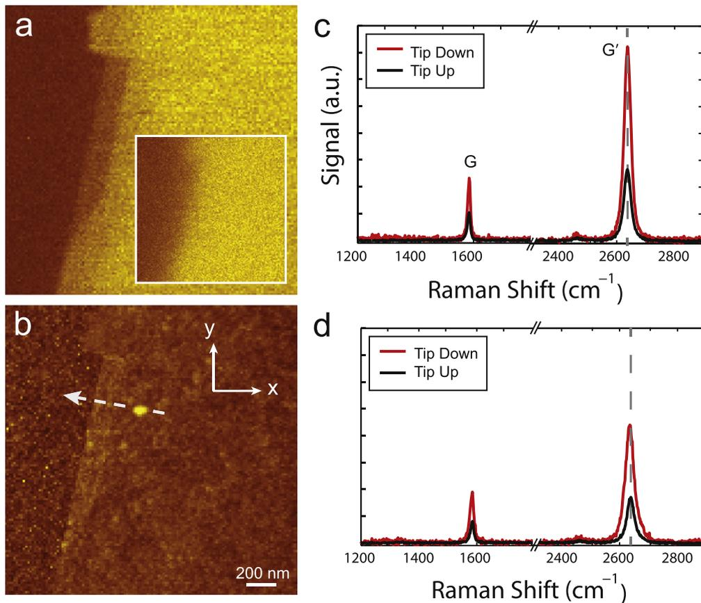
**Figure 1.** TERS characterization of a graphene sample. (a) TERS image of the G' band. Inset: confocal image of the same area scaled in intensity by  $\times 2$  compared to the TERS image. (b) Simultaneously acquired topography of the flake in (a). The white arrow indicates the location, taken tail to head, of the hyperspectral linescan. (c), (d) Spectra with (red) and without (black) the tip away from and near the particle.
