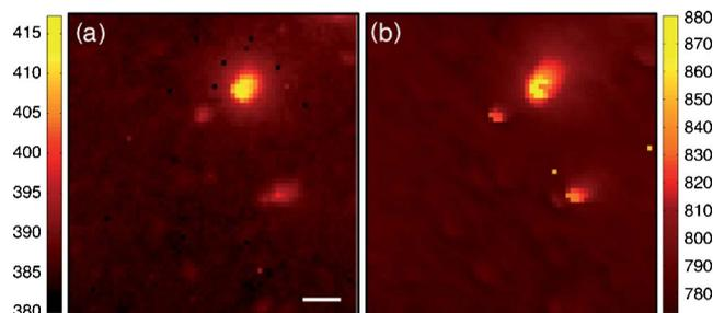
Fig. 3. (Color online) Spatial maps of the center frequencies of  $m=2$  and  $m=3$  cavity modes. (a)  $m=3$  mode, (b)  $m=2$  mode. Scalebar:  $2\ \mu\text{m}$ .
