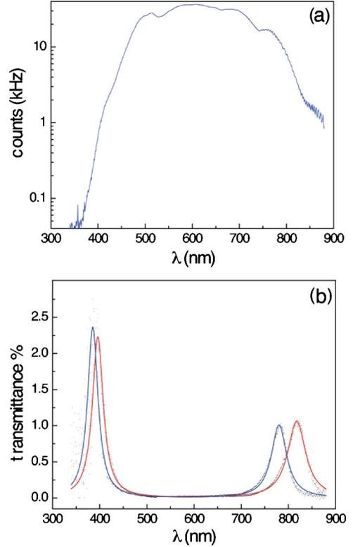
Fig. 2. (Color online) (a) Spectrum of the white-light source employed in the experiments. (b) Cavity transmittance spectrum in the absence [black (blue online)] and presence [gray (red online)] of a single gold nanoparticle. The solid lines are Lorentzian fits to the experimental data (black dots).
