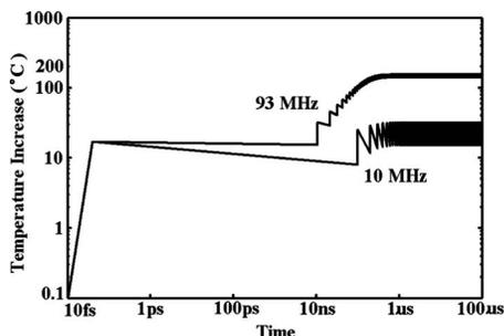
Fig. 7. Temperature increase at the laser focus induced by 800 nm, 27 fs laser pulses in water. The 93 MHz pulse train used in our experiment can create as high as a  $150^\circ\text{C}$  temperature increase. In the contrast, a 10 MHz pulse train can only provide about a  $20^\circ\text{C}$  temperature increase at the laser focus.
