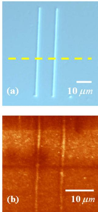
Fig. 2. (Color online) (a) DIC image of laser modified lines on the surface of Balafilcon A. Several Raman spectra were taken along the dashed line. (b) Confocal luminescence image of these lines (the wavelength detection window is 695–705 nm).
