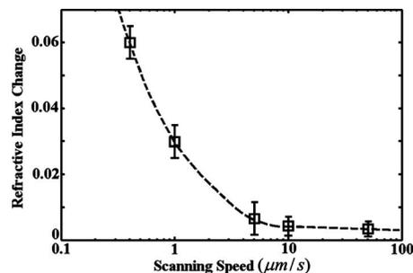
Fig. 8. Refractive index changes of the hydrogel polymers as a function of laser scanning speed.
