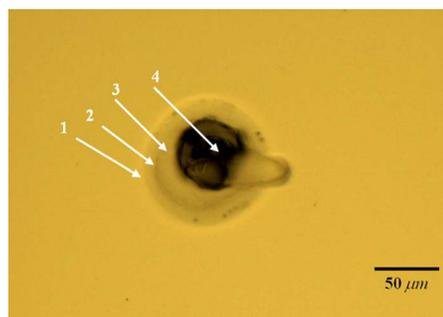
Fig. 5. (Color online) Bright field image of a damage spot in Balafilcon A with high femtosecond laser irradiance. Raman spectra of four points of the damage spot from its periphery (point 1) to its center (point 4) were measured.
