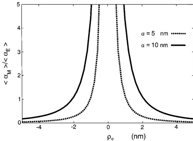
Fig. 4. Inverse ratio ( $\langle \alpha_M \rangle / \langle \alpha_E \rangle$ ) as a function of the radial coordinate  $\rho_0$  of a quantum dot with  $a = 5$  nm and  $a = 10$  nm. In a length interval of a few nanometers, the magnetic dipole absorption rate is stronger than the electric dipole absorption rate. The ratio is largely independent of N.A., but a large N.A. is required for a good signal-to-noise ratio.  $\lambda = 532$  nm,  $f_0 = 1$ .
