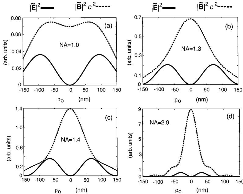
Fig. 2. Electric field  $|\tilde{\mathbf{E}}|^2$  (solid curves) and magnetic field  $|\tilde{\mathbf{B}}|^2$  (dashed curves) of a focused azimuthally polarized beam evaluated in the focal plane as a function of the radial coordinate  $\rho_0$  for numerical apertures  $N.A. = 1.0, 1.3, 1.4, 2.9$ . The electric field is zero at the center, whereas the magnetic field strength increases as the N.A. becomes larger. The wavelength is  $\lambda = 532$  nm; the filling factor is  $f_0 = 1$ .
