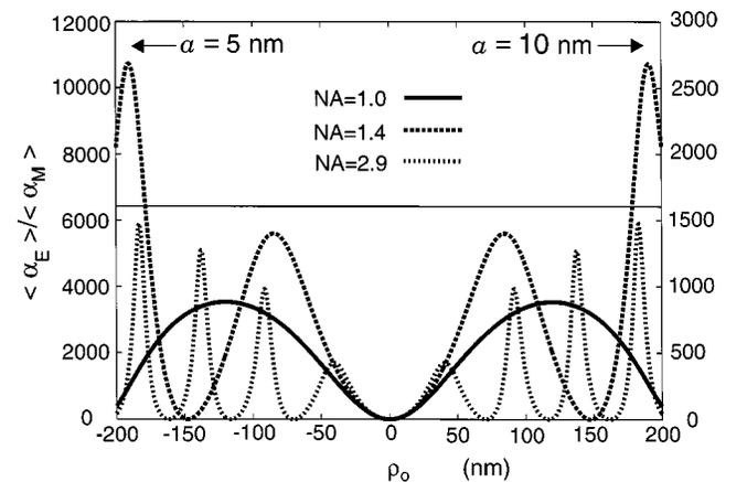
Fig. 3. Ratio of the magnetic dipole and electric dipole absorption rates ( $\langle \alpha_E \rangle / \langle \alpha_M \rangle$ ) as a function of the radial coordinate  $\rho_o$  of the quantum dot. The left (right) vertical axis corresponds to quantum dot radius  $a = 5$  nm ( $a = 10$  nm). The ratio corresponding to plane-wave excitation is indicated by the horizontal line.  $\lambda = 532$  nm,  $f_o = 1$ .
