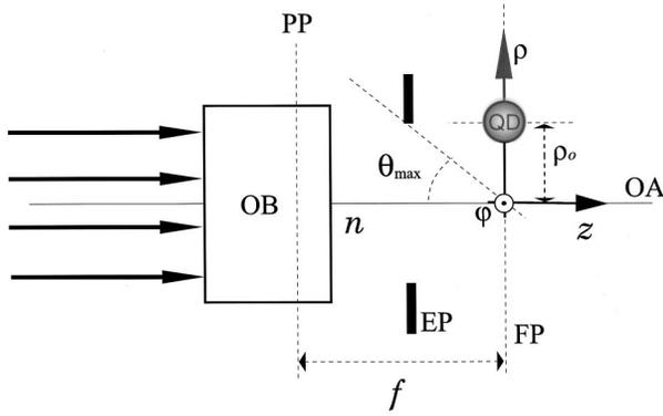
Fig. 1. Excitation of a spherical quantum dot (QD) with a focused azimuthally polarized beam. An objective (OB) with focal distance  $f$  [distance between rear principal plane (PP) and focal plane (FP)] and numerical aperture  $N.A. = n \sin \theta_{\max}$  focuses an incoming azimuthally polarized beam through an exit pupil (EP) along the optical axis (OA) on the focal plane. The quantum dot is located in the focal plane at  $\mathbf{r}_0 = \rho_0 \mathbf{n}_\rho$ .
