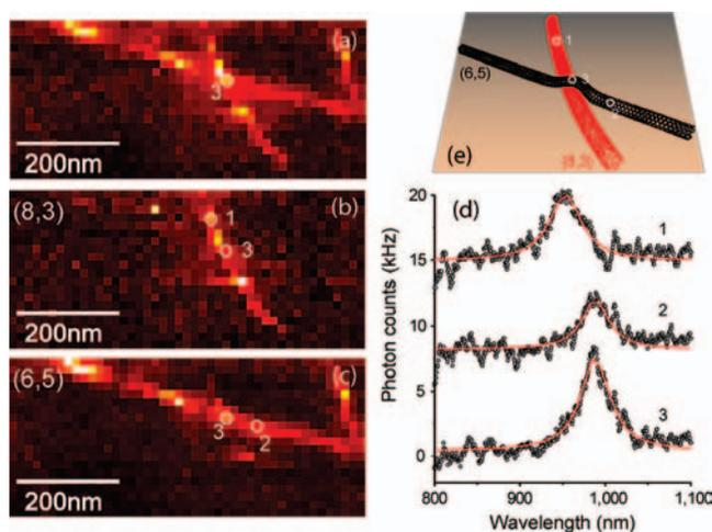
**Figure 3.** Near-field PL image of two intersecting nanotubes obtained by measuring spectra at each pixel representing the integrated intensity within selected spectral windows. (a) Total intensity. The intensity integrated from 915 to 945 nm is shown in (b) and from 970 to 1010 nm in (c). (d) Spectra taken at the pixels marked by white circles and numbers 1–3 in (a), (b), and (c). (e) Simplified schematic of the intersecting nanotubes.
