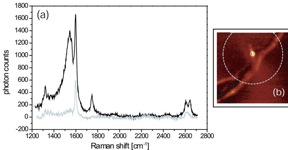
Fig. 3. (a) Raman spectra detected on top of the bright feature marked in (b): With metal tip (black curve) and without tip (grey curve). (b) Near-field Raman image showing the intensity of the G band. Scan area  $400\text{ nm} \times 400\text{ nm}$ . The white circles indicate the areas probed in the near-field (solid line) and farfield (dashed line).
