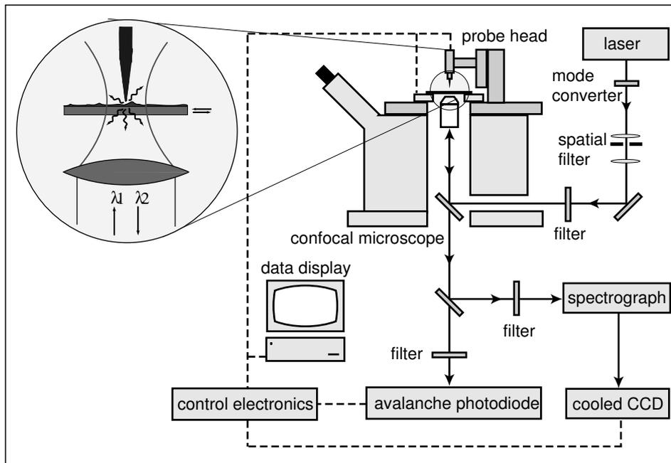
Fig. 1. Schematic of the experimental setup. A sharp metal tip is positioned above a carbon nanotube sample and centered into a tightly focused radially polarized laser beam. An optical scan image is obtained by laterally scanning the sample using a (x,y)-scan stage. The optical signal is detected either after spectral filtering by an avalanche photodiode (APD) or by a combination of a spectrograph and a CCD.
