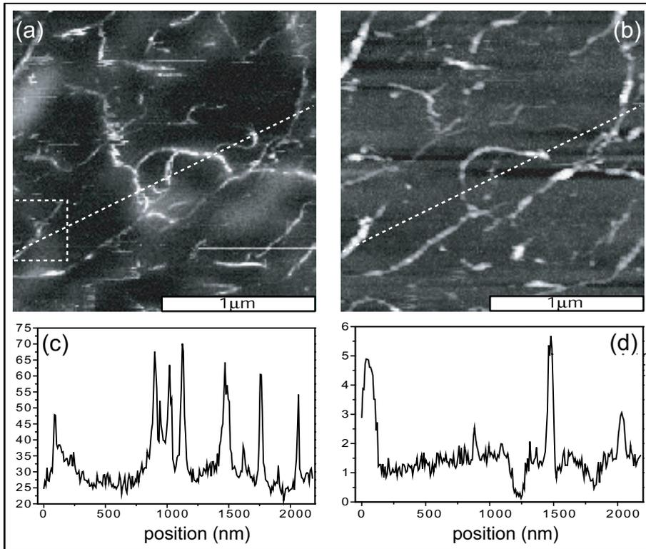
Fig. 2. Simultaneous near-field Raman image (a) and topographic image (b) of SWNTs on glass. Scan area  $2 \times 2 \mu\text{m}^2$ . The Raman image is acquired by detecting the intensity of the G band upon laser excitation at 632.8 nm. (c) Cross section taken along the indicated dashed line in the Raman image. (d) Cross section taken along the indicated dashed line in the topographic image. Vertical units are 1000 photon counts per second for (c) and nanometer for (d).
