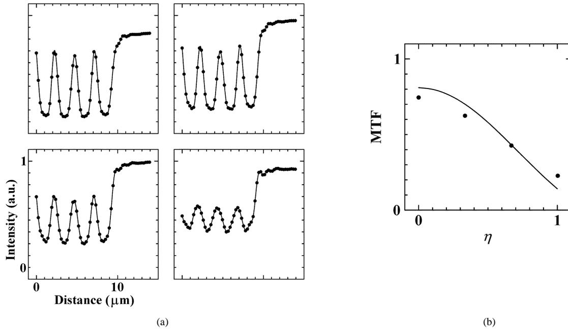
Fig. 6. Through substrate imaging of a silicon IC using an AMOS-200 IC failure analysis system demonstrating the improvement in longitudinal resolution. (a) Line scans of periodic  $0.4 \mu\text{m}$  periodic structures with defocus steps of  $1 \mu\text{m}$ . (b) Modulation transfer function showing close to diffraction limited performance.
