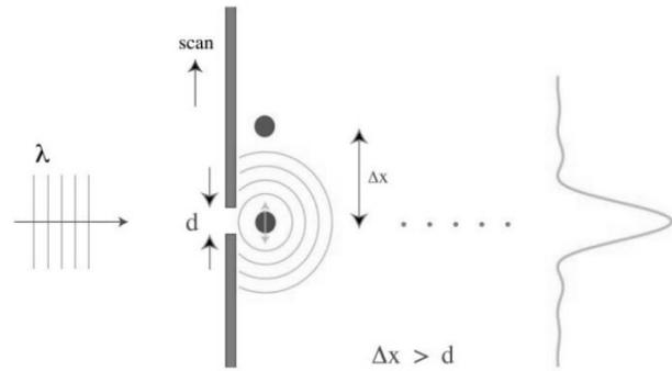
Fig. 2. Schematic of aperture scanning near-field microscopy.
