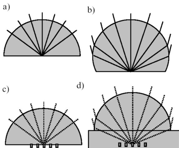
Fig. 3. Solid immersion lens configurations. In (a), a hemispherical lens increases resolution by  $\sim n$ . (b) A Weierstrass optic, or super-SIL, has a resolution increase of  $\sim n^2$ . Two types of imaging modes, surface solid immersion microscopy (c) and subsurface SIM in (d).
