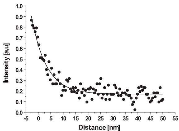
Fig. 3. Tip-sample distance dependence of the fluorescent emission. The experimental data (circles) can be fitted with a single exponential with a decay constant of approximately 6 nm (solid curve).
