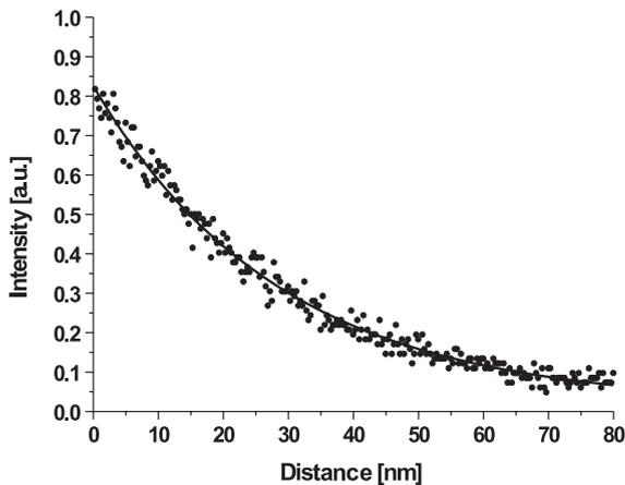
Fig. 7. Tip–sample distance dependence of the white-light continuum (500–700 nm) generated at the apex of a sharp metallic tip. The experimental data (squares) can be fitted with a single exponential with a decay length of 30 nm (solid curve).
