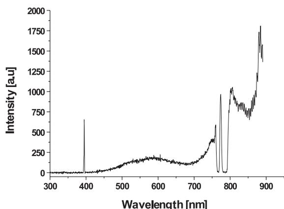
Fig. 4. Emission spectrum of gold tip excited at 780 nm by the longitudinal field in focused Gaussian laser spot on a glass cover slip. A second-harmonic peak situated at 390 nm and a broad band continuum is readily seen. The shape of the spectrum around 780 nm is due to the laser notch filter.
