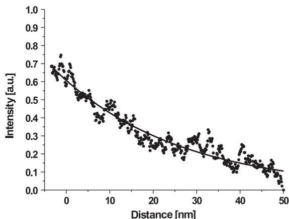
Fig. 5. Tip-sample distance dependence of the second-harmonic signal generated at a sharp gold tip. The experimental data (circles) can be fitted with a single exponential with a decay constant of 28 nm (solid curve).
