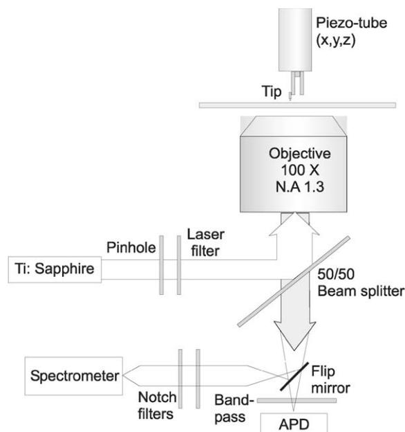
Fig. 1. Experimental set-up. A Ti:sapphire laser is spatially and spectrally filtered and focused on a glass cover slip. A gold tip is held above the focal spot. The emission of the sample, respectively of the tip, is collected by the same objective and is focused on either an avalanche photodiode (APD) or a spectrometer.
