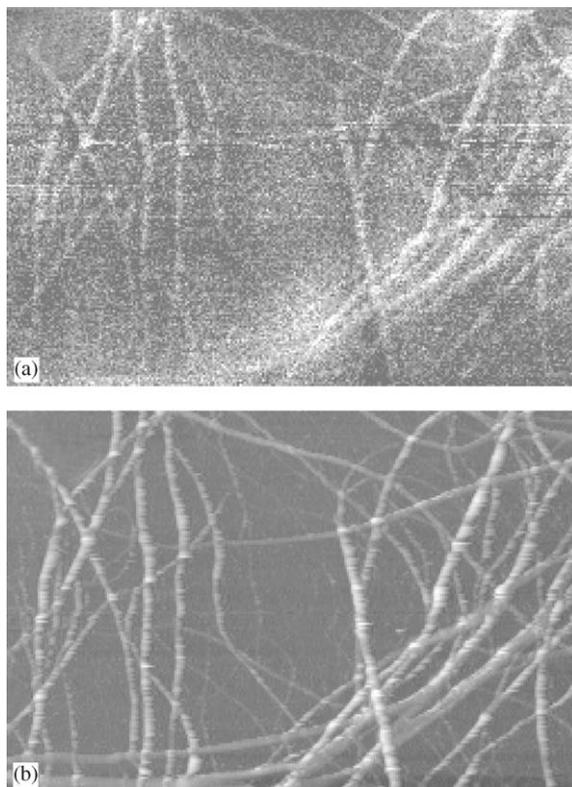
Fig. 2. (a) Fluorescent emission image of *J*-aggregates. The optical resolution is  $\sim 25$  nm. (b) Topographical image. The aggregates form an interwoven mesh of tubulus. Images are  $3 \mu\text{m} \times 2 \mu\text{m}$ .
