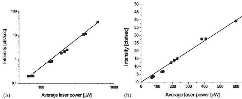
Fig. 6. Power dependence of the visible (a) and near infra-red (b) parts of the spectrum (Fig. 4). The visible depends quasi-quadratically on the average excitation power (slope 2.3, log–log scale) whereas the infra-red part increases linearly with excitation (slope 0.06).
