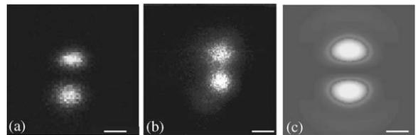
Fig. 8. Spatial distribution of second-harmonic (a) and photoluminescence (b) acquired with different tips. (c) Calculated distribution of longitudinal fields in the focus of a Gaussian beam (NA = 1.3). Scale bar: 250 nm.
