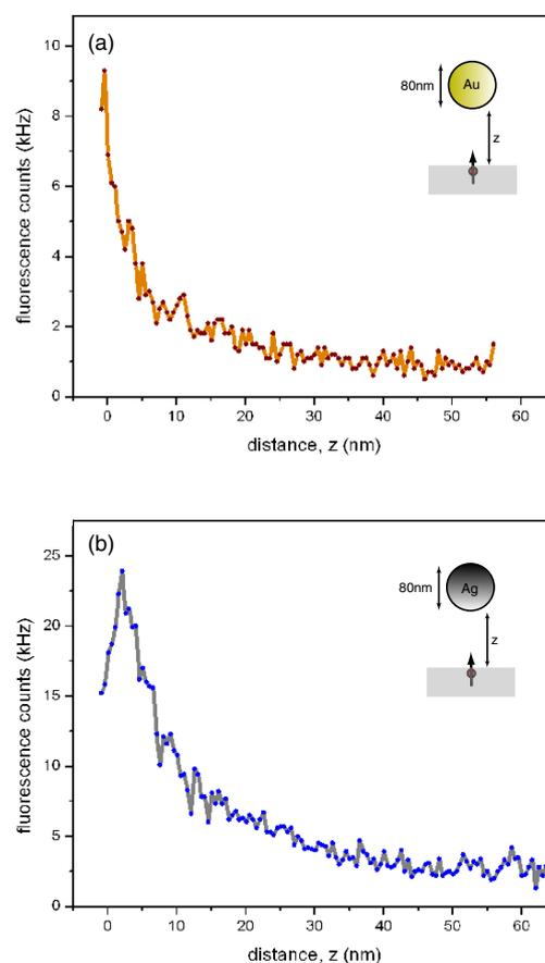
**Figure 3.** Single molecule fluorescence rate as a function of particle-sample distance for (a) an 80 nm gold particle and (b) an 80 nm silver particle. At short distance the fluorescence enhancement drops due to nonradiative decay (energy transfer from the excited molecule to the particle). Both gold and silver particles yield similar enhancement at the excitation wavelength of  $\lambda = 637$  nm.
