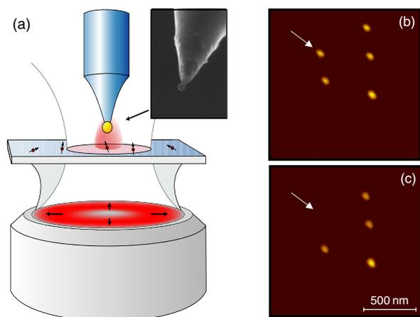
**Figure 1.** (a) Schematic diagram of the experimental setup. A radially polarized laser beam is focused on the surface of a glass coverslip with well-separated single dye molecules. The fluorescence is monitored as a function of the proximity of a single gold or silver nanoparticle antenna attached to the end of a glass tip. The inset shows an SEM image of a nanoparticle tip. (b) Topographic image of a sample with isolated gold particles before picking and (c) after picking.
